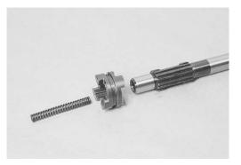
3. Drive the dog pin out of the clutch dog shifter.
