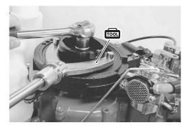
5. Remove the flywheel from the crankshaft using the special tool.
