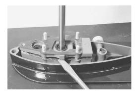
15. Pull out the driveshaft with the driveshaft support housing and remove the washer.
