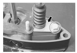
8. Remove the propeller shaft bearing housing.
